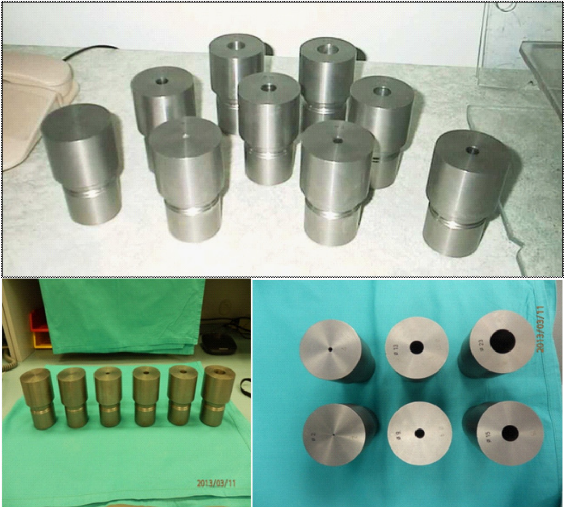
Figure 3: Interchangeable collimators (an orifice with different diameters, varying from 5 to 40 mm, in steps of 5 mm).
