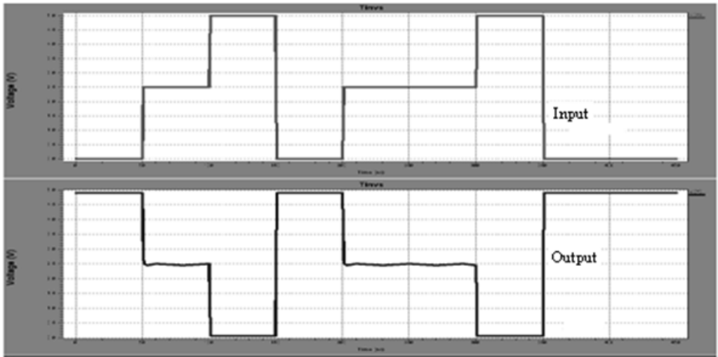
Figure 7.1: (a) T-Simple Inverter circuit (b) Lay out for Simple T-Interter, (C) Waveforms for T-Simple Inverter
